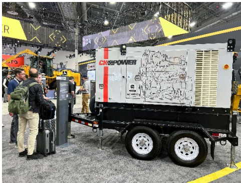
Photo Caption 2 : CK Power's 60–70kW generator prototype, powered by the JD4 engine, is showcased at the John Deere Power Systems booth, demonstrating innovation and OEM partnership.
